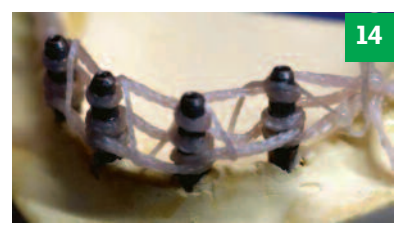
Fig. 9: Tests were conducted in the harshest conditions by subjecting the distal extension of a sample CST-type implant to a cantilever flexion test.
