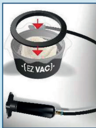
6- Clamp EZ-VAC system with membrane and cover
