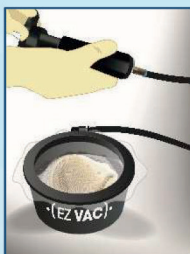
8- Using the pump, evacuate the air to press the mesh against the model and close valve
